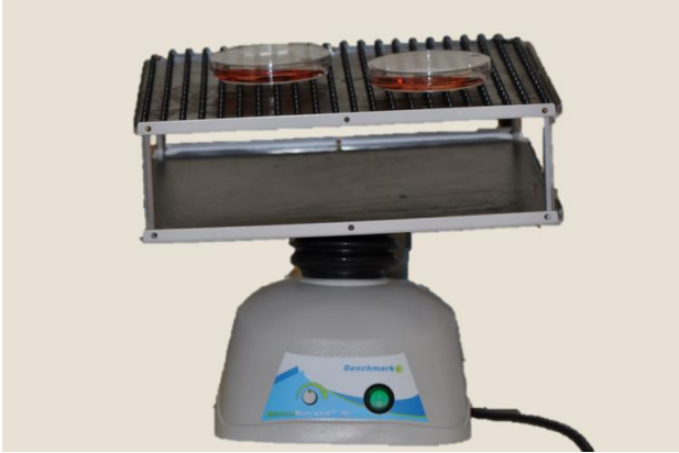
Figure 3-4: Rocker setup including petri dishes with corneas. Note the 6 degree incline that aided in bathing the corneas eight times per minute. The rocker was placed in the CO 2 incubator.
